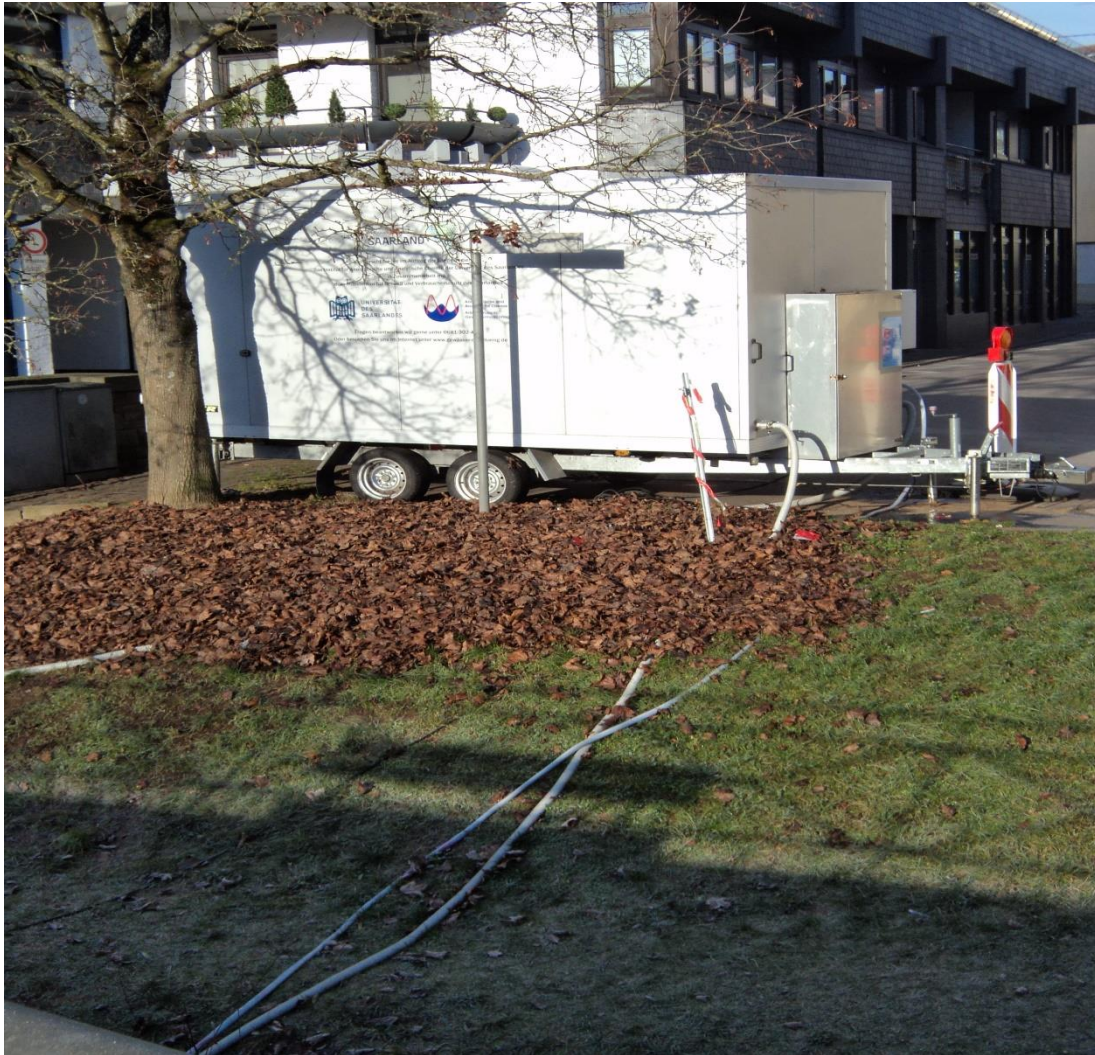
108 109 Fig. 1. Water monitoring station (Saardand lands, Germany) (Photo credit: Olena Mitryasova)
